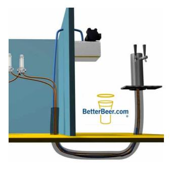
The Line Chiller (aka Power Pack or Glycol Deck) is responsible for keeping beer cold inside the trunk line. It is important to know that the Line Chiller keeps cold beer cold, it doesn't make warm beer cold. The beer that enters the trunk should be cold, thus the importance of a cold walk-in fridge. Just to be clear, cold is defined as 3°C (38°F).
