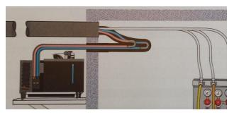
The supply and return lines leave the deck and go into the fridge, close to where the trunk line exits the fridge. The supply and return lines enter the trunk while it is still inside the fridge to ensure that there are no warm (or non-chilled) areas of the beer lines.
