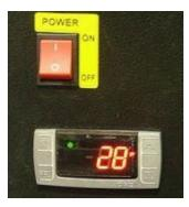
On the front of the deck is a LED display that will show the temperature of the glycol inside the bath. This number should be between 28 and 33. Typically, there is a six-degree swing between the bath temperature and the tap temperature. If the bath is at 28, the tap temp will usually be 34. The Molson Sub Zero system and some larger, high powered systems are the exceptions to this rule, but for the most part, you are looking for 28-33 on the reading.
